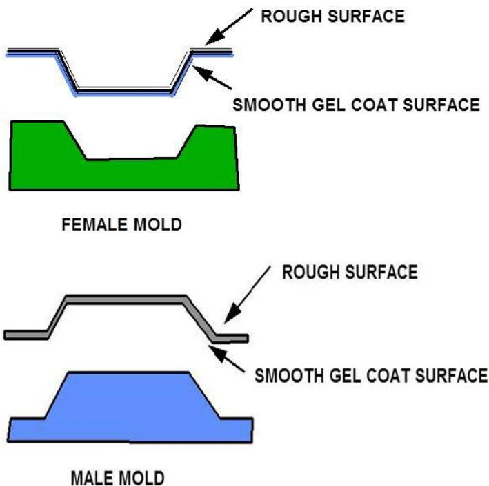
For very short production runs (less than 10 parts), temporary molds can be made from wood, foam, clay or plaster. These molds are economical and can be fabricated quickly, which will allow inexpensive prototype parts to be fabricated. For larger volume production, molds are typically made with fiberglass. These molds have a life expectancy of 10+ years and 1000+ cycles. Fiberglass molds are inexpensive and usually only cost 6 to 10 times the price of the part.
